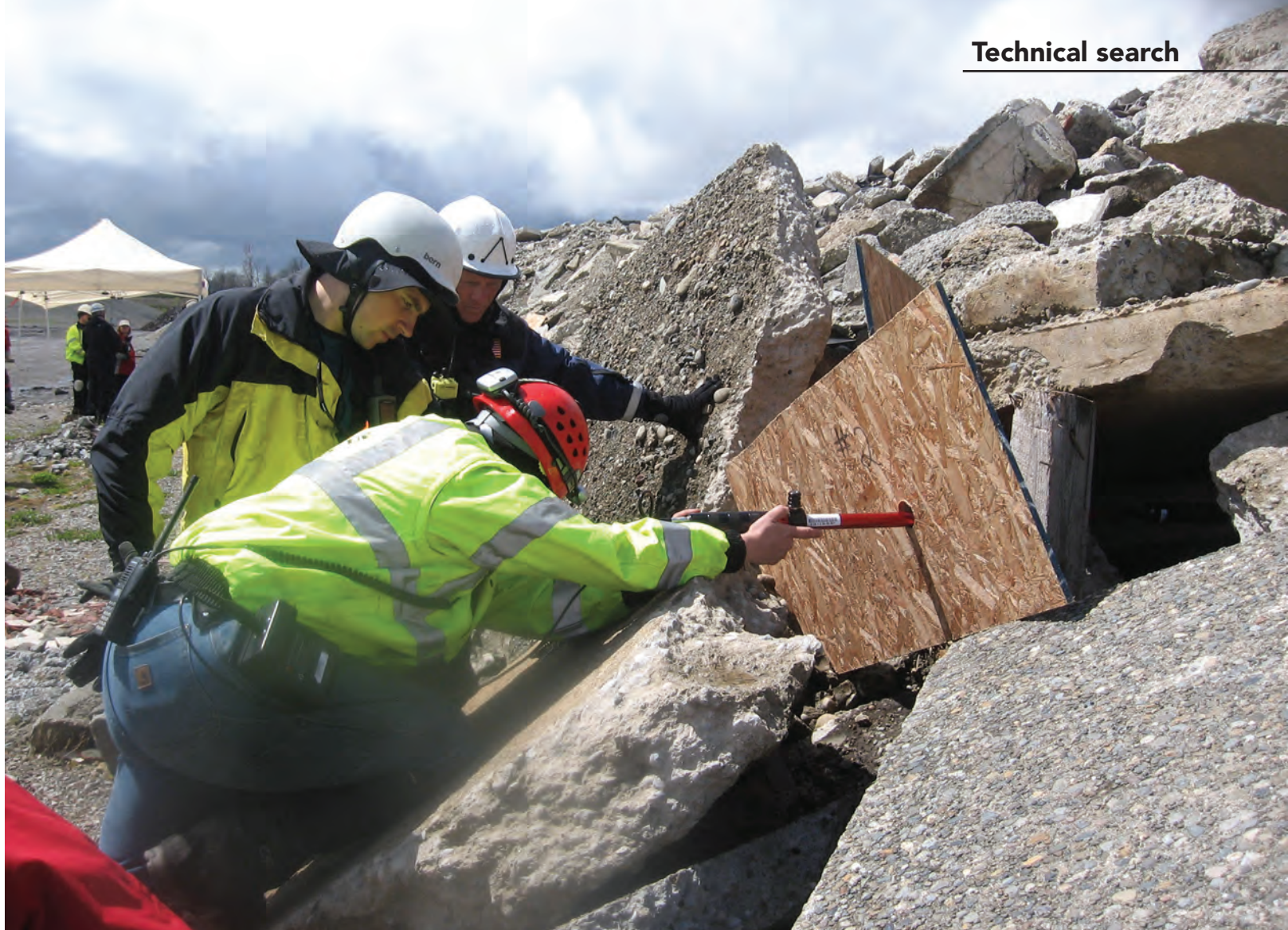
Search and rescue volunteers practicing with a telescoping camera to explore pile of rubble
